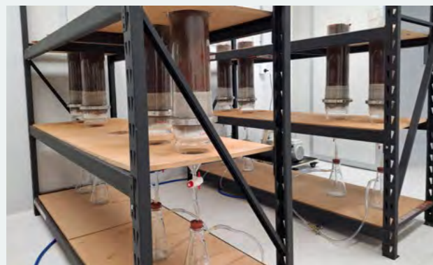
Leaching columns used in the project
